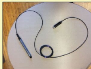
Figure 5 (Left): HOBO MX pressure transducer. Used to measure stream stage.
