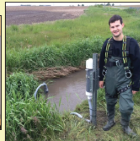
Figure 5 (Left): HOBO MX pressure transducer. Used to measure stream stage.
