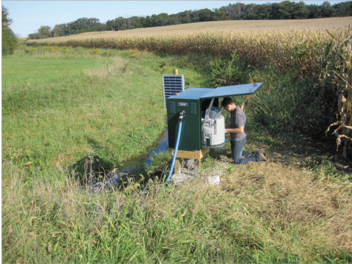
Figure: The FTS monitoring station setup for another project in the Lake Bloomington watershed.
