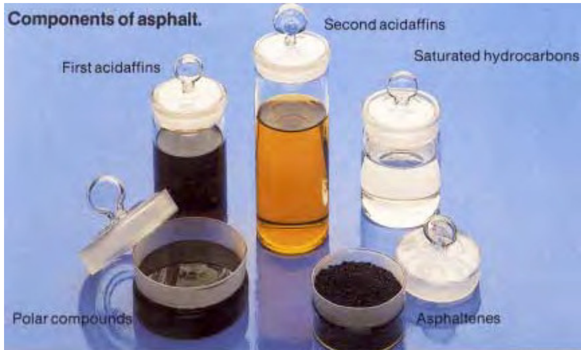
Figure 1. Asphalt Binder Fractions, Asphaltenes and Maltenes.
