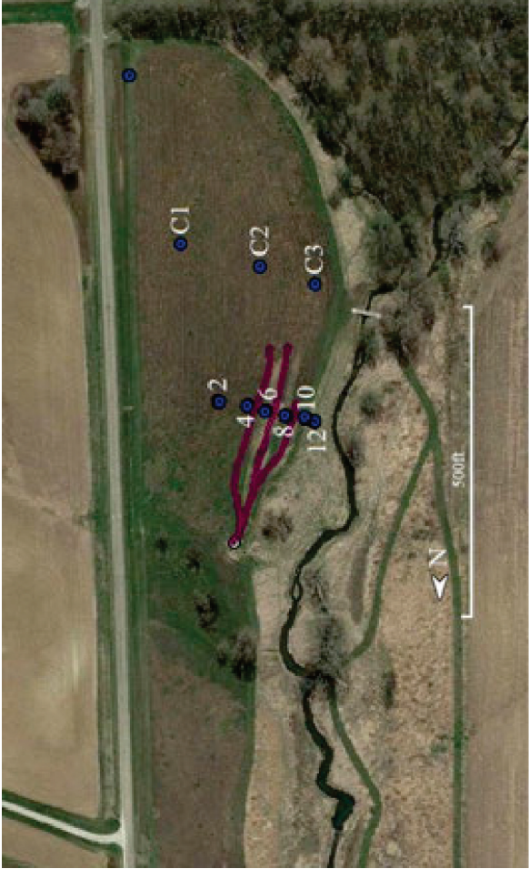
Figure 1: Study site; with diversion box (white), diversion wells (blue 2, 4, 6, 8, 10, 12), reference wells (C1, C2, C3), and redirected subsurface tiles (red)
