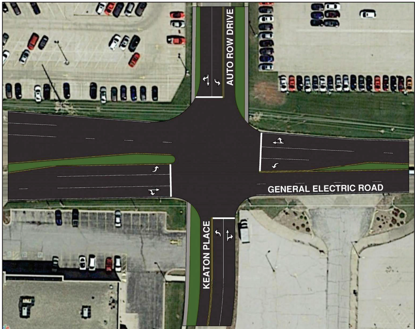
Figure 20 - General Electric Road / Keaton Place Intersection Concept
