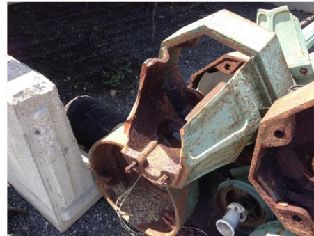
Figure 7 – Shows the damaged pole salvaged from the Bloomington Country Club Place project with a broken base and center bracket.
