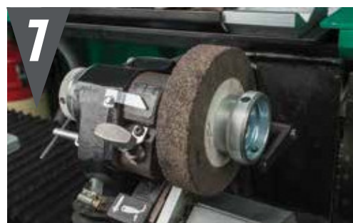
ROBUST GRINDING HEAD & RELIEF ASSEMBLY
