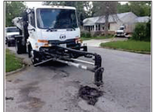
Example of pothole spray injection equipment
