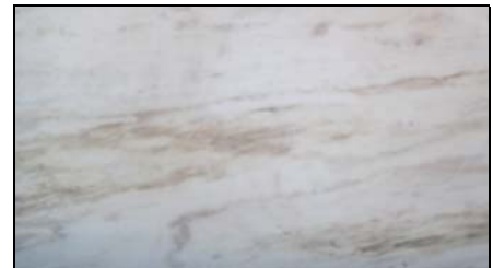
Marble – Typically fine grained and able to be highly polished; it has a wide range of colors and patterns; used for steps and stoops, statuary and fine masonry.
