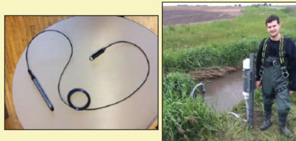
Figure 5 (Left): HOBO MX pressure transducer. Used to measure stream stage.
