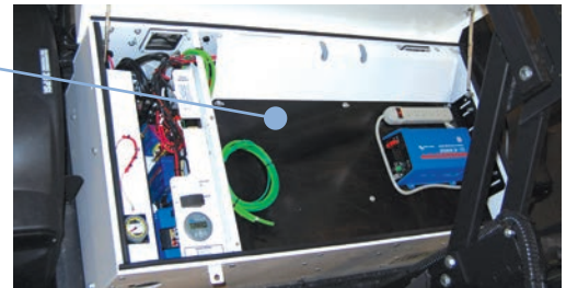
Battery box interior (optional inverter shown)
